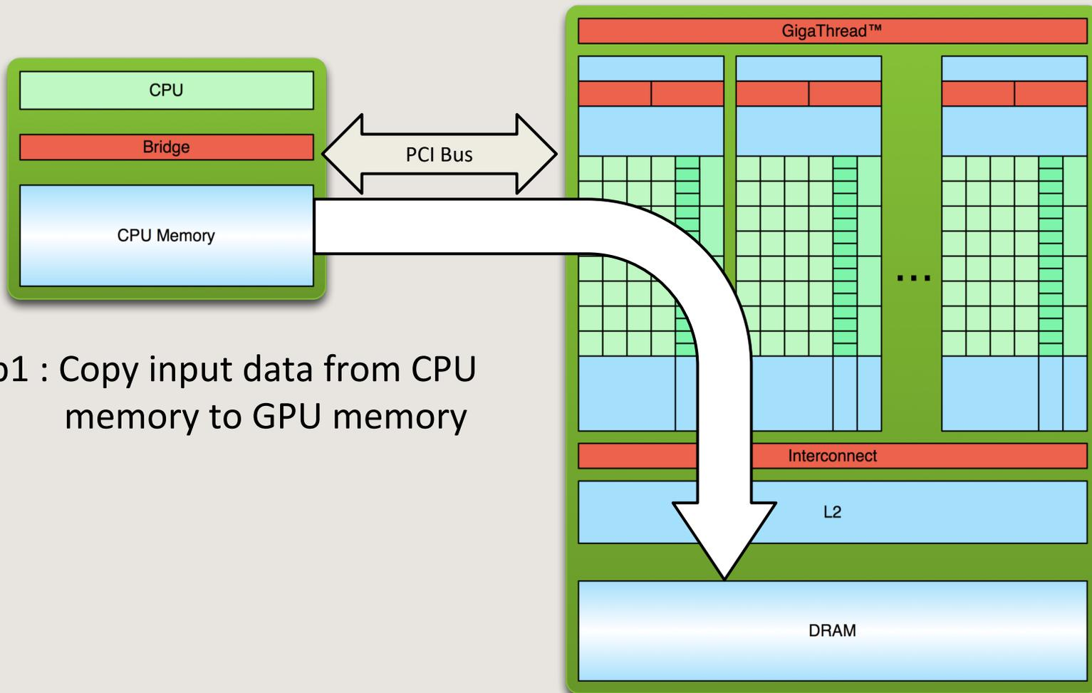
Step1 : Copy input data from CPU memory to GPU memory
