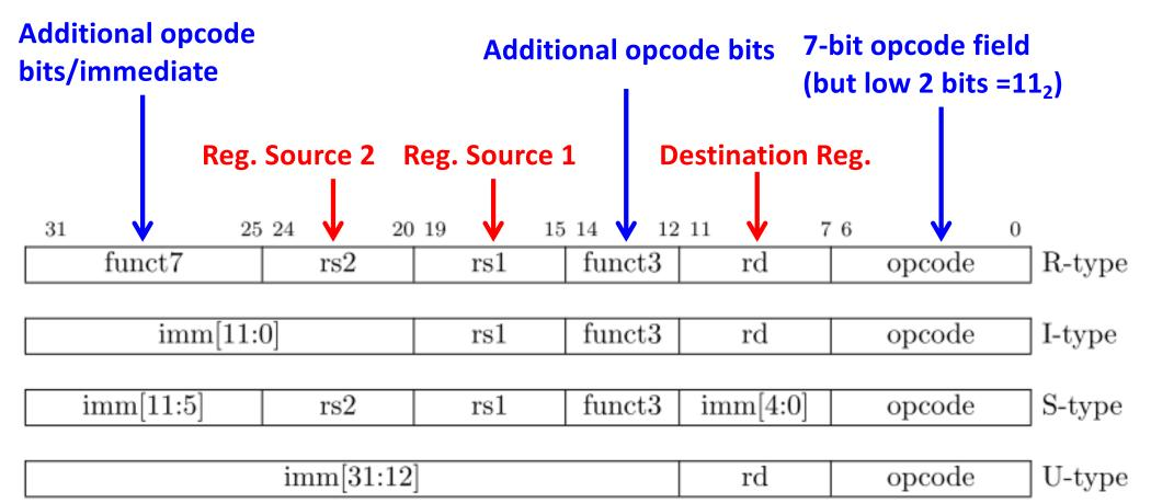
Aligned on a four-byte boundary in memory. There are variants! Sign bit of immediates always on bit 31 of instruction. Register fields never move.
