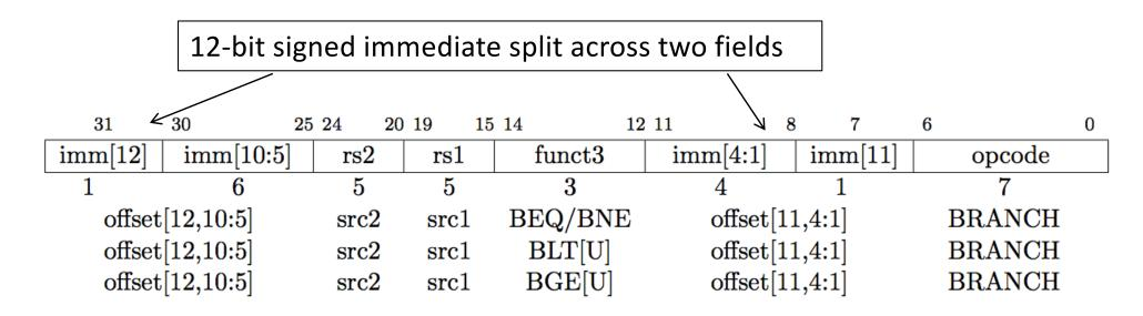
Branches, compare two registers, PC+(immediate<<1) target (Signed offset in multiples of two). Branches do not have delay slot
