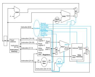
Review lecture slides 31 – 67 of Chapter 04 (<u>https://passlab.github.io/ITSC3181/notes/Chapter04\_Processor.pdf#page=31</u>) about the datapath and control of a single-cycle RISC-V processor design.
