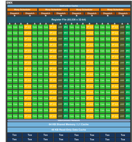
SMX: 192 single-precision CUDA cores, 64 double-precision units, 32 special function units (SFU), and 32 load/store units (LD/ST).
