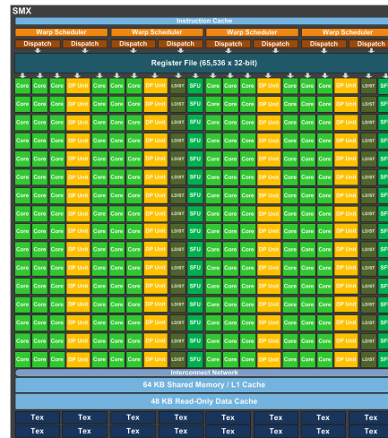
SMX: 160 single-precision CUDA cores, 64 double-precision units, 32 special function units (SFU), and 32 load/store units (LD/ST).
