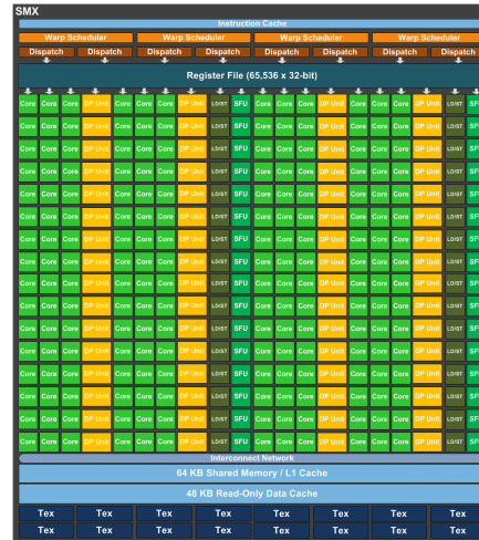
SMX: 152 single-precision CUDA cores, 64 double-precision units, 32 special function units (SFU), and 32 load/store units (LD/ST).
